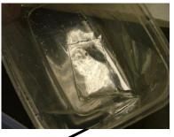
Spraying EtBr destroyer sprayer 3 times (about 0.9 ml) again and placed for 30 min
